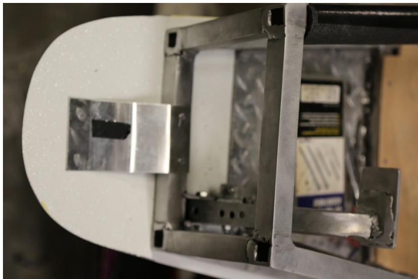
Front-end protection - 8" x 8" Frame Members (top view)
