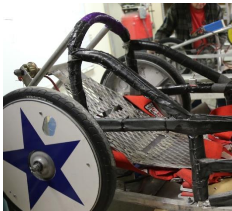
Roll cage with bracing front and rear
