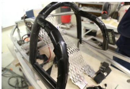
Padding installed around the roll cage tubing
