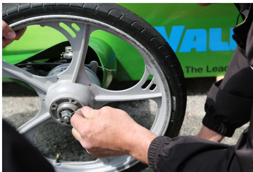
Cotter pin inserted into the wheel nut for safety
