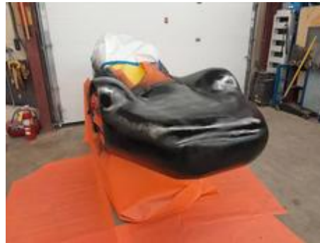
We are now on to the painting of the A107, we have chosen a color shift paint for the car. To start we had to apply a base coat of gloss black, for the best look when we get to the actual final color shift paint.
