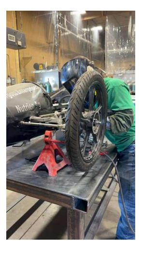
Kris got the old brake caliper brackets taken off and new brackets designed and made for them.
